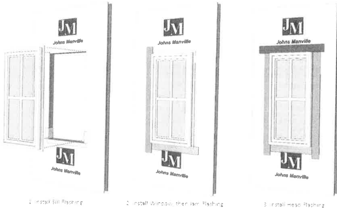
FIGURE 4: TYPICAL PENETRATION FLASHING DETAIL - FLANGED
